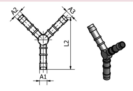
Ext. Hose Diameter A1 = 13Ext. Hose Diameter A2 = 13Ext. Hose Diameter A3 = 13L2 = 65
